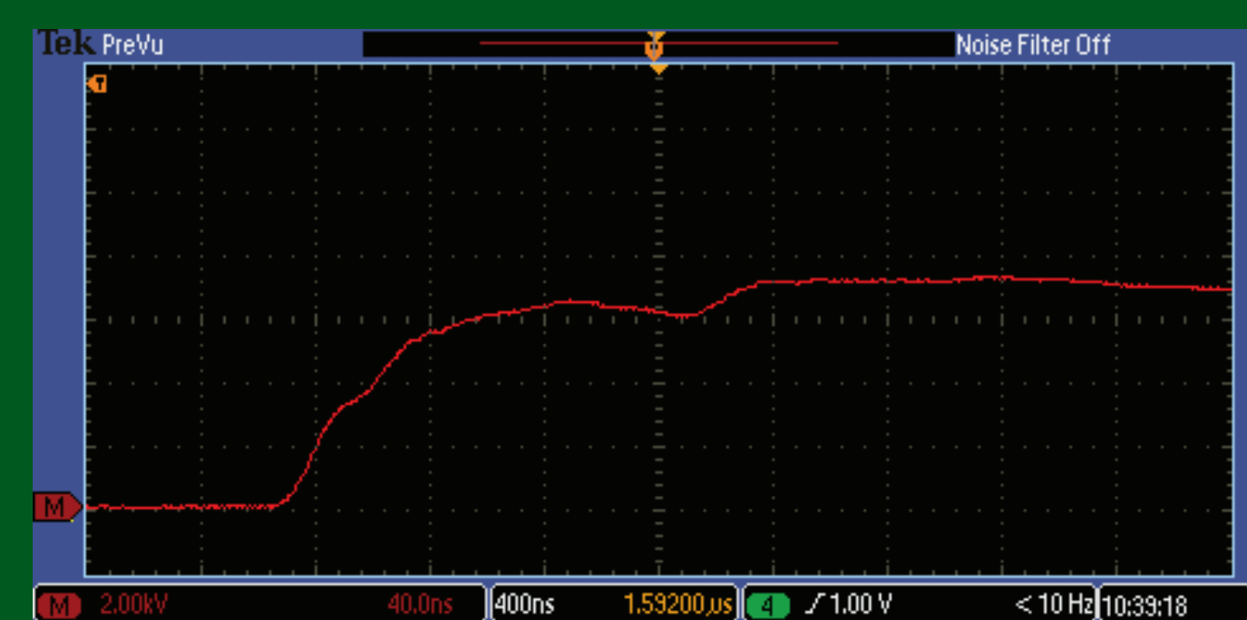
Expanded scale ~ 40 ns rise time Slew rate in excess of 100 kV/ms!
