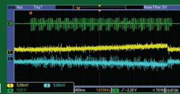
Differential probe measurement of integrator channel crosstalk error.
