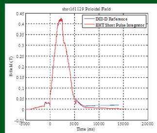
DIII-D vs EHT Poloidal Field measurement.
