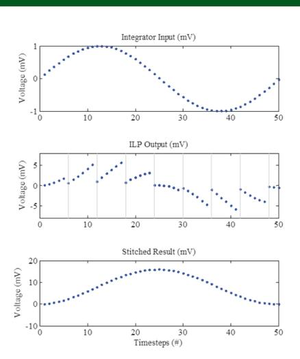
Simulated integrator input (top), raw integrator output (middle), and stitched data (bottom).
