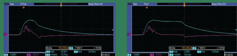
Output voltage (blue) and output current (pink) measured with 1:4.5 voltage divider and current transformer for a 10 kV pulse of 80 ns (left) and 184 ns (right) into a DBD
