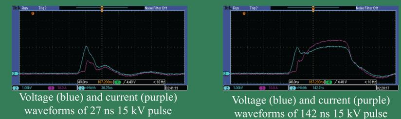
Voltage (blue) and current (purple) waveforms of 27 ns 15 kV pulse
