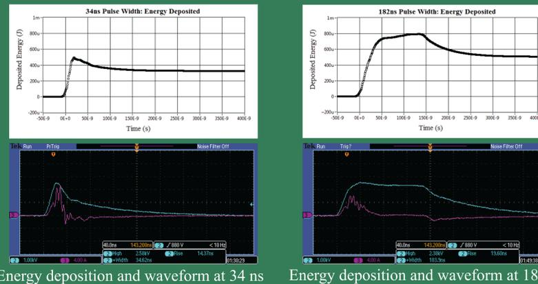
Energy deposition and waveform at 34 ns Energy deposition and waveform at 182 ns
