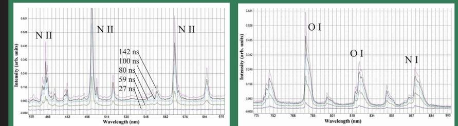
Some high intensity lines are only visible at pulse widths >27 ns (left plot), while other lines of similar intensity are represented at all pulse widths (right plot).
