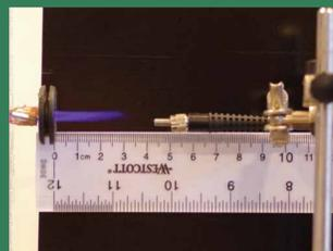
Plasma plume and spectrometer fiber.
