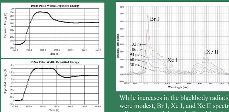
106 ns and 132 ns pulses deposited 1.2 mJ and 1.4 mJ into the plasma, respectively.
