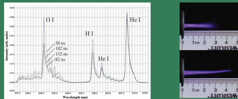
Operation at different pulse widths clearly shows intensity variation of O and H lines, but not He lines
