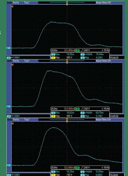
Output voltage pulses at 66 (top), 74 (middle), and 80 kV (bottom).
