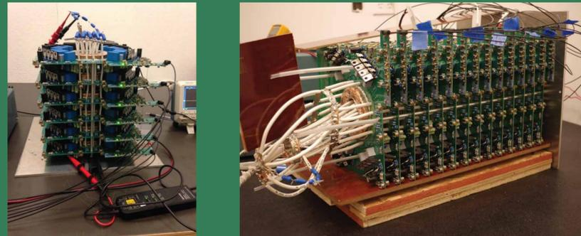
Left: 10 kV inductive adder. Right: 20 kV inductive adder.
