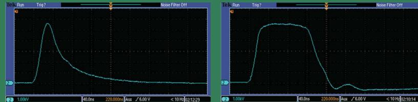
40 kV pulse with 20 ns rise and 40 ns FWHM (Left) and 130 ns FWHM (Right).
