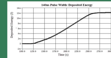
A plot of energy deposited into the arc with respect to time (left) is consistent with the expectation of a constant power, and helps validate other power measurements
