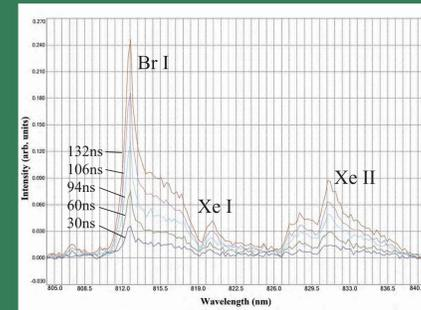
While increases in the blackbody radiation were modest, Br I, Xe I, and Xe II spectral lines increased dramatically with pulse width. This indicates potential utility of nanosecond pulsers in exomer production
