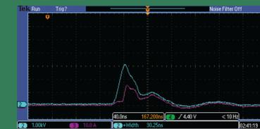
Voltage (blue) and current (purple) waveforms of 27ns 15kV pulse
