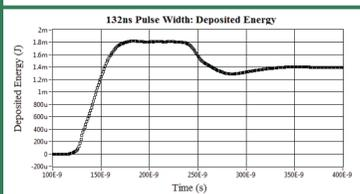
106ns and 132ns pulses deposited 1.2mJ and 1.4mJ into the plasma, respectively.
