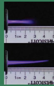
Gas flow decreased from 7.4 - 1.5 sL/min. Maximum jet length was at 2.4 sL/min
