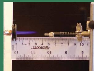
Plasma plume and spectrometer fiber.
