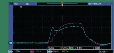
Voltage (blue) and current (purple) waveforms of 142ns 15kV pulse
