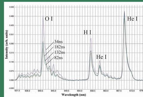
Operation at different pulse widths clearly shows intensity variation of O and H lines, but not He lines
