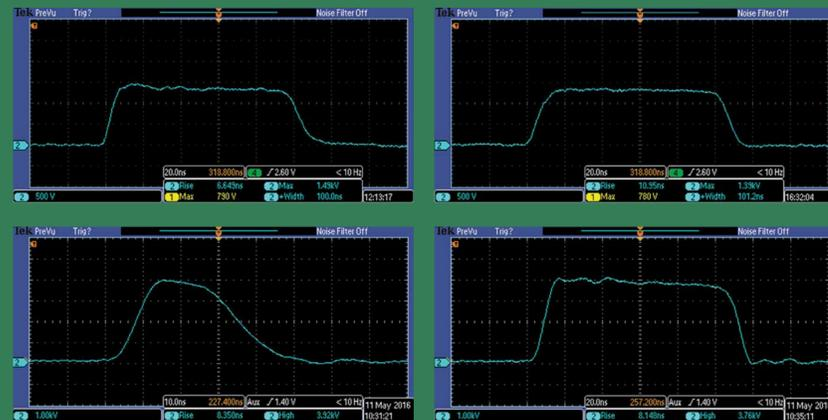
Top Left: 10 kV - 100 ns pulse into 50 load with 6.6 ns rise time. Top Right: 10 kV - 100 ns pulse into 25  $\Omega$  load with 11 ns rise time. Bottom: 20 kV, 51 ns (left) and 110 ns pulse widths into 50  $\Omega$  load with 8.4 ns rise.
