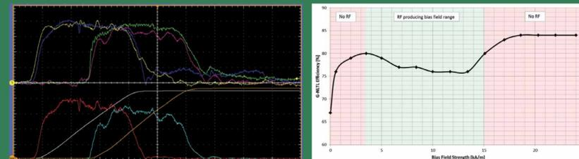
Left: Signals for G-NLTL single shot efficiency driving 52  $\Omega$  load at a bias field of  $\approx$  17 kA/m. Input voltage (yellow), input current (blue), load voltage (purple), load current (green), instantaneous input power (red), instantaneous output power (cyan), total input energy (white), and total energy delivered to the load (orange). Efficiency is  $\approx$  83 %. Right: Coaxial NLTL broadband efficiency vs bias field strength.
