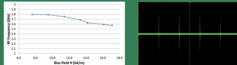
Left: NLTL RF output frequency as a function of magnetic bias field. Right: CVP output with 12.6 [kA/m] bias field. Burst of 4 pulses at 100 kHz. Horizontal scale 5  $\mu$ s/div, vertical scale 3333 V/div.
