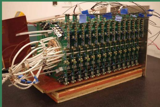
20 kV inductive adder capable of 50  $\Omega$  driving.
