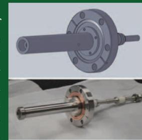
SPG: CAD drawing and completed vacuum hardware.
