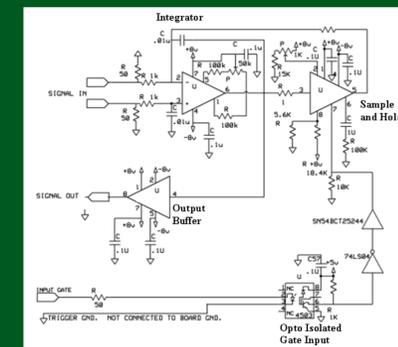
Pre-Phase I, High gain integrator board and circuit diagram. The simple design provides a low cost option for the integrators with performance realized through careful board design and component selection. The pre-Phase I design is suitable for applications requiring integration times for several seconds. The Phase I program will incorporate new features to dramatically reduce droop and overall drift over much longer periods appropriate for long pulse applications
