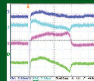
Pre-Phase I program integrator drift measurement (Left). Integrator output for the Phase I design showing similar drift over a longer time period (Right). New methods for drift reduction are currently under investigation.
