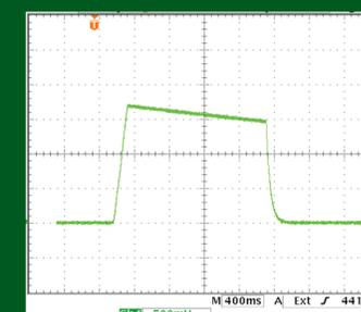
Pre-Phase I program integrator droop measurement (Left). Integrator output for the Phase I design showing little droop over 10s of seconds (Right).
