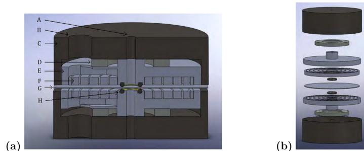
FIGURE 2: Solidworks model of proposed valve, (a) Cross sectional view (A=Gas inlet, B=BNC inlet, C=Upper iron casing, D=Permanent cylindrical magnet, E=Aluminum solenoid plate, F=5-turn pancake solenoid, G=Aluminum/Steel moving disk, H=Buna-N O-ring) and (b) disassembled view.
