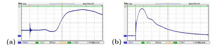
FIGURE 4: (a) Output of fiber optic displacement sensor using 1000 V pulse suggesting a 70  $\mu$ s rise time, and (b) voltage signal over a 5 m $\Omega$  resistor suggesting 12 kA of current.
