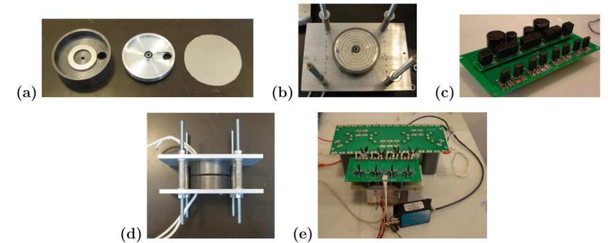
FIGURE 3: (a) Individual valve components, (b) assembled configuration of valve upper half, (c) High Current Adapter on IGBT board, (d) fully assembled moving disk valve, and (e) complete experimental set-up.
