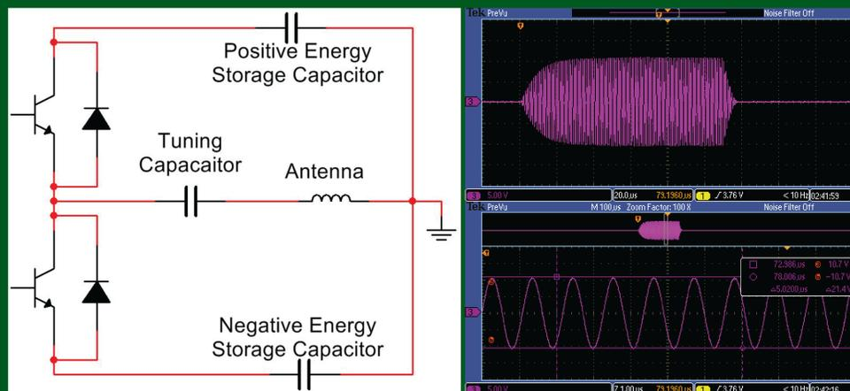
Left: Circuit diagram showing the EPS antenna resonant half bridge power supply. Right: Antenna current profile for 100  $\mu\text{s}$  shot: Full waveform (Upper) and zoomed in scale (Lower). The current in the antenna is 1.7 kA.
