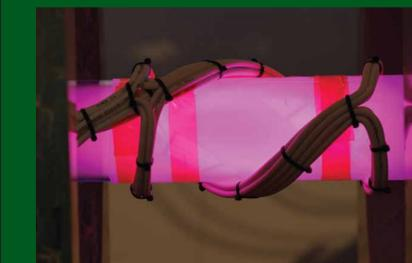
The high density/flow rate EPS with hydrogen plasma under the antenna.
