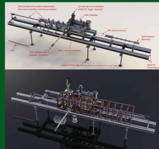
Schematics of the material science chamber and EPS showing the key sections and transfer arms (upper) and the magnet sizes and locations (lower).
