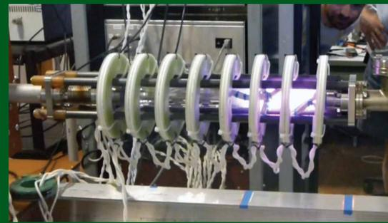
Laboratory testing of Phase II EPS generating hydrogen plasma prior to transfer to HIT group.
