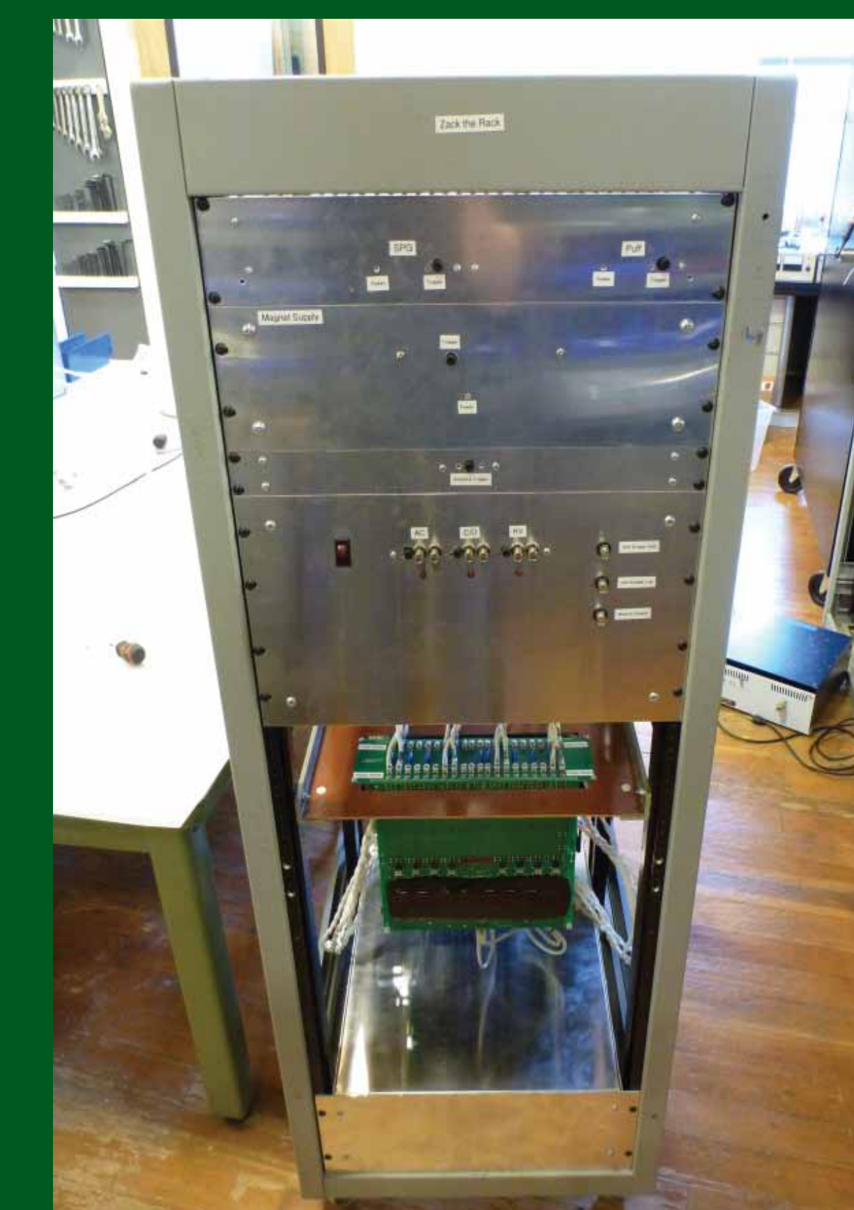
Phase II, Half Bridge Series Resonant Converter. Utilized for plasma source antenna and magnet drivers. Capable of 1 MHz Switching at high pulsed power levels (> 5 MW Peak).
