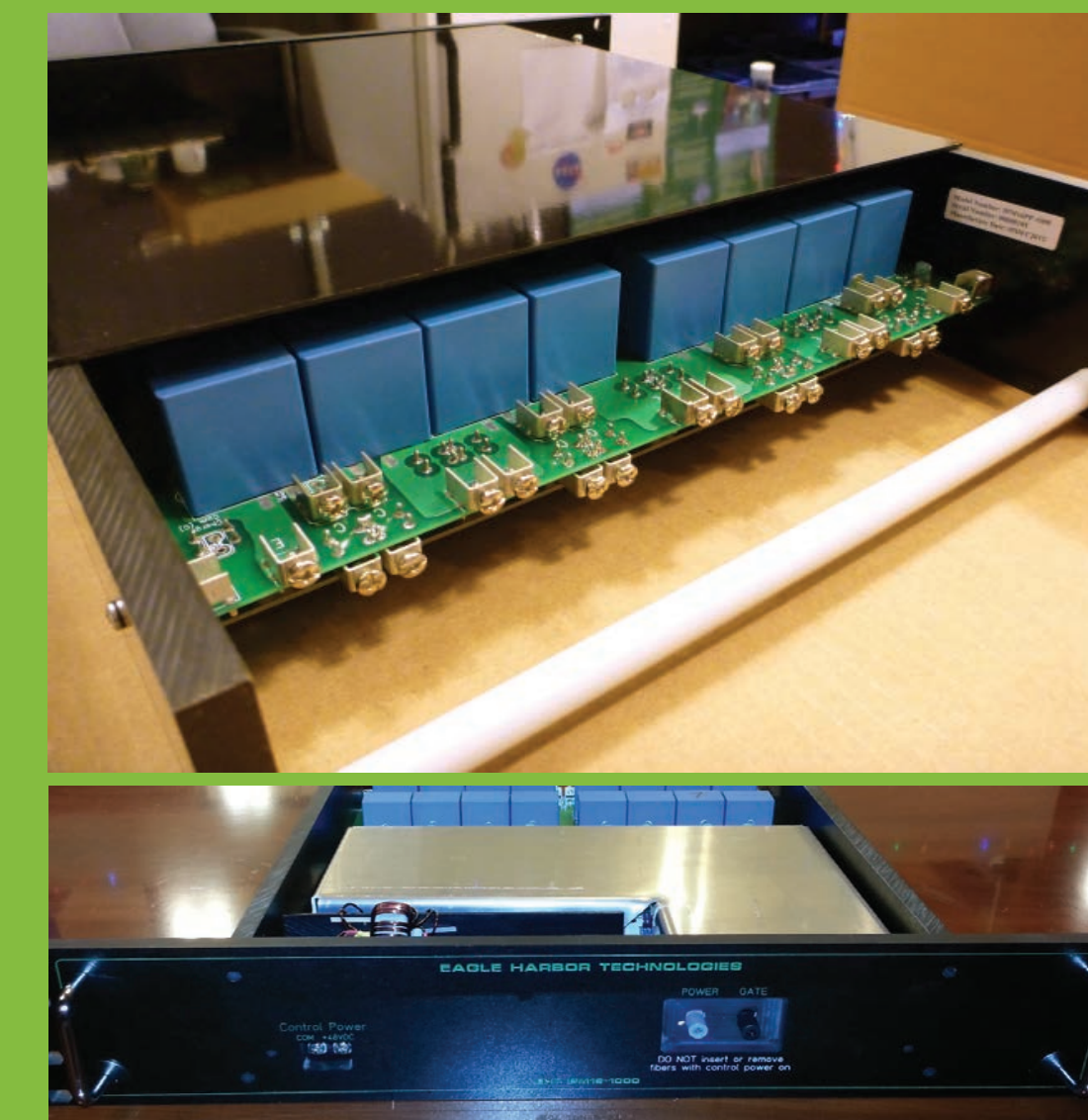
Left: IGBT-16P module. Right Upper: High current connectors. Right Lower: 2U Rack Mountable Module: 8" x 11" x 2.5"
