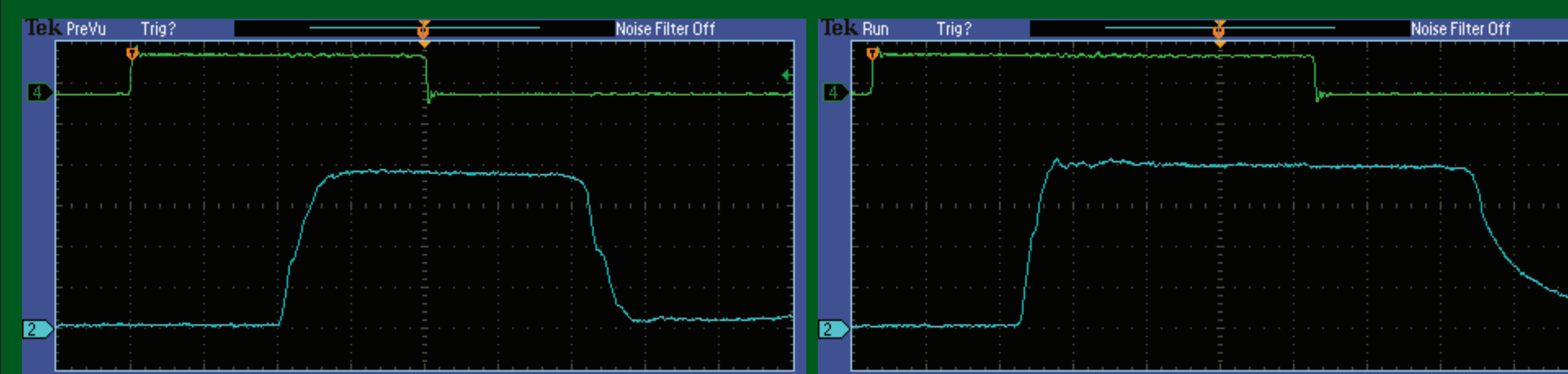
Left: Load voltage for 400 A, 400 ns pulse. Middle: Load voltage for 150 A, 600 ns pulse. Right: 12 module stack using IPM-4P.
