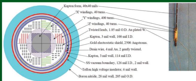
Cross section of the RPPL internal magnetic probe showing the selected materials and thicknesses. (Inset) Photo of one three-axis magnetic probe constructed at RPPL.
