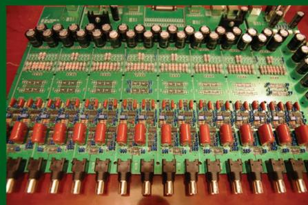
Sixteen channel, short pulse integrator developed for validation platform experiments through DOE SBIR Phase I/II.
