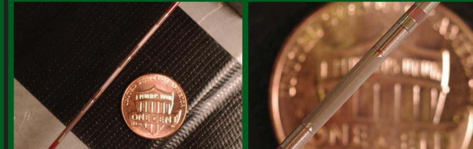
(Left) Three-channel, three-axis probe (nine coils total) on polyimide tube made using 3D printing techniques. (Right) Zoomed in photo of the probe showing a single three-axis channel with 25  $\mu$ m trace widths visible.
