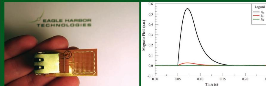
(Left) Three-axis surface probe with RJ-45 connector made using flexible PCB printing techniques. (Right) Magnetic field inside a pulsed solenoid measured off-axis using the three-axis surface probe.
