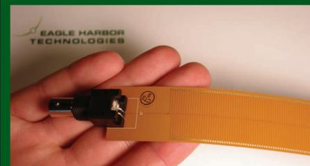
(Upper Left) Rogowski coil with BNC connector made using flexible PCB printing techniques. (Lower Left) Rogowski coil shown in coiled configuration. (Lower Right) Current in a pulsed solenoid magnet as measured by the flexible Rogowski coil.
