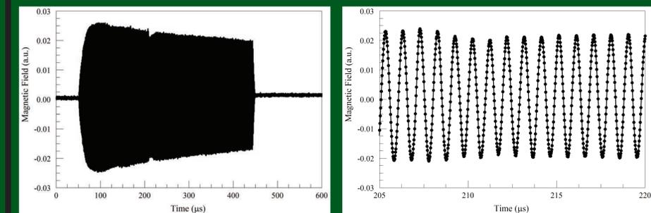
(Left) Internal magnetic field in an RF inductive plasma source (no plasma present) as measured with the 3D printed magnetic probe. The antenna frequency is 1 MHz. (Right) Zoomed in magnetic field trace showing that the individual field oscillations are cleanly resolved. The signal was digitized at 50 MS/s.
