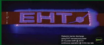
Dielectric barrier discharge using EHT nanosecond pulser. 20 ns pulse width @ 20 kV continuous operation @ 5 kHz rep rate.
