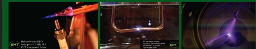
Left: EHT nanosecond pulser driving an atmospheric DBD-based plasma pencil made with flowing helium gas. Middle: Water plasma discharge driven by EHT nanosecond pulser. Right: Pseudospark generated in low pressure argon background (~200 mTorr). To create the pseudospark, the pulser produced 30 kV, 80 ns pulses at 200 Hz during CW operation.
