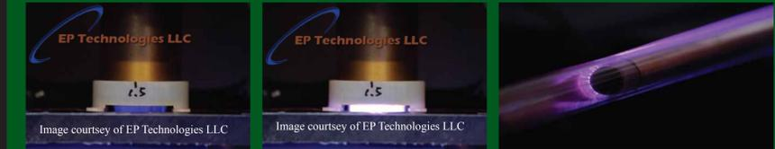
EHT nanosecond pulser driving dielectric barrier discharges (DBD). The DBD driver for EP Technologies operated at 20 kV at 100 Hz (left) and 10 kHz (middle) for plasma medicine applications. At right, a 1 m long DBD-based plasma wand for atmospheric drag reduction demonstrating the capability of driving high capacitance DBDs.
