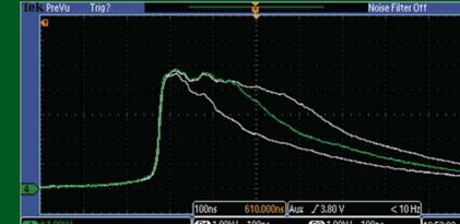
Compressed 12 kV pulses with variable pulse widths.
