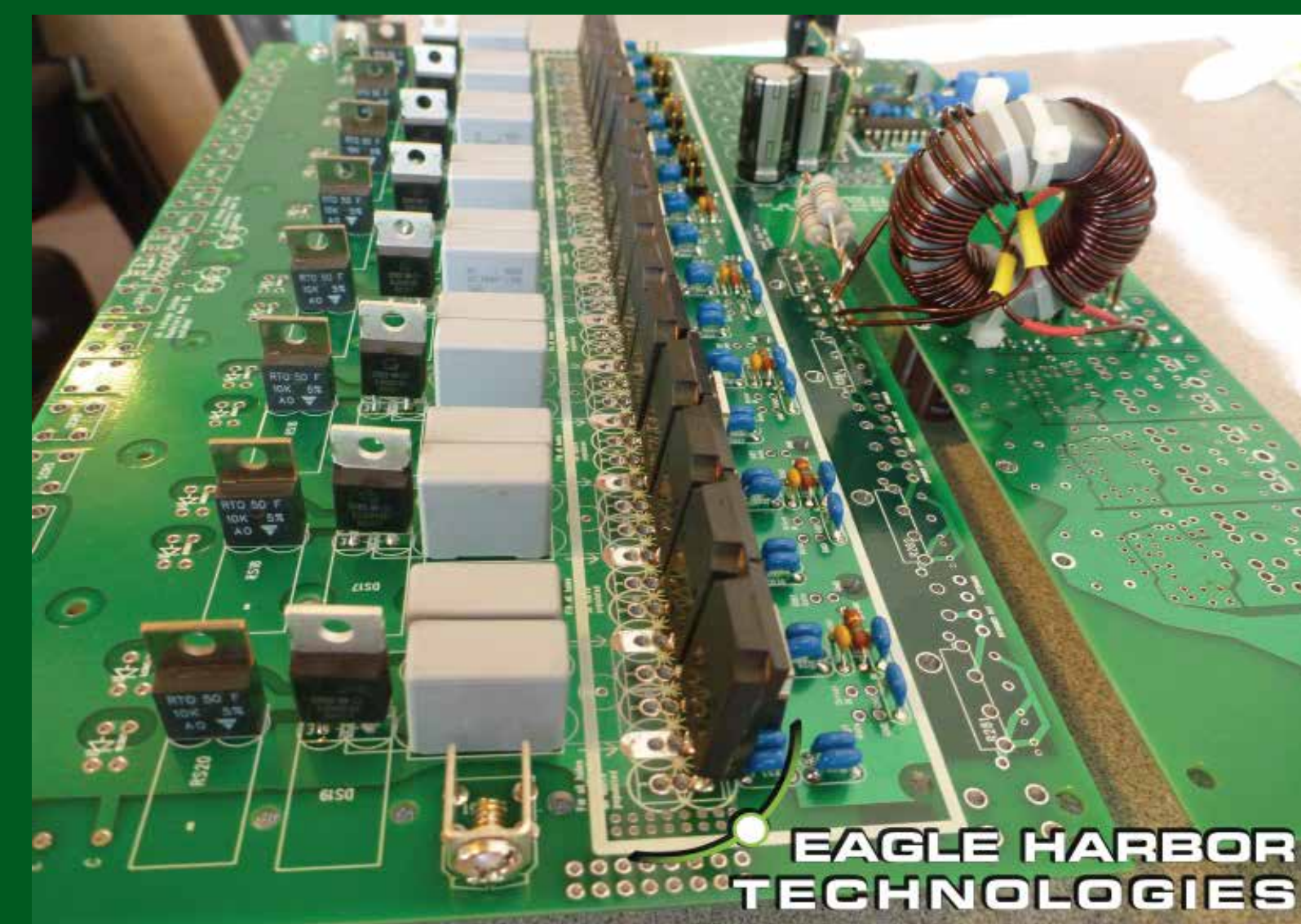
Left: IGBT-16P module. Right Upper: High current connectors. Right Lower: 2U Rack Mountable Module: 8" x 11" x 2.5"
