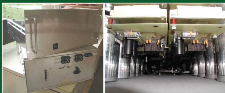
Left: The front and back of the SPA modules currently used at HIT. Right: Inside the SPA module showing the capacitors, IGBTs, and driver boards.
