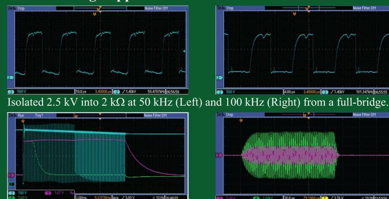
Isolated 2.5 kV into 2 k $\Omega$  at 50 kHz (Left) and 100 kHz (Right) from a full-bridge.
