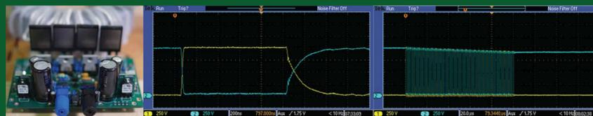
Left: Test stand to characterize IGBTs and SiC MOSFETs. MOSFET switching (CH1 (yellow):  $V_{load}$  and CH2 (blue):  $V_{DS}$ ). Middle: Single 1  $\mu$ s pulse switching 40 A/device at 1 kV. Right: 100 pulses at 1 MHz switching with 50% duty cycle 40 A/device at 1 kV. The voltage drop by the end of the 100 pulses is due to energy being drained from the capacitor
