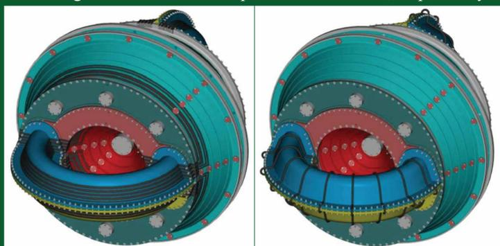
The HIT-SI3 chamber and injectors showing the voltage coil (left) and the flux coil (right).
