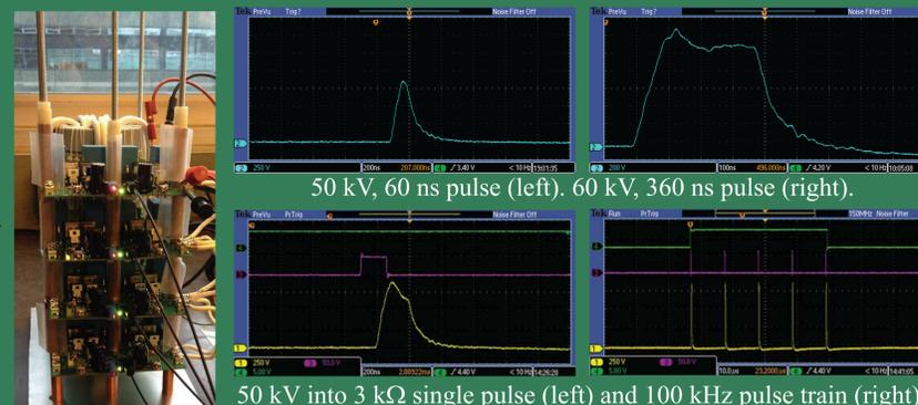
High voltage nanosecond pulser test setup to demonstrate high voltage 100 kHz frequency
