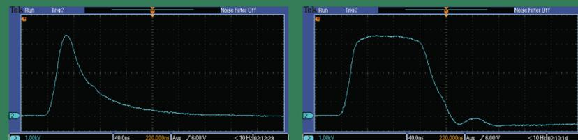
$T_{rise} \approx 20$  ns, Pulse width  $\approx 40$  ns FWHM      $T_{rise} \approx 20$  ns, Pulse width  $\approx 130$  ns FWHM
