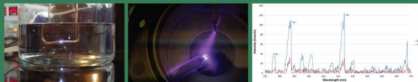
Underwater discharge (left). Pseudospark in low pressure xenon (middle). APPJ plume spectra demonstrating the effect of varying the pulse width (right)
