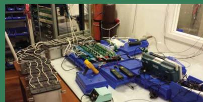
High current switching test set-up
