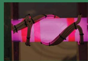
High power inductive plasma generation using high current resonant tank network
