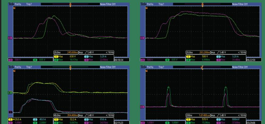
NLTL input and output for 40 ns (top right) and 120 ns pulse (top left). Measurement of efficiency (bottom left). High frequency burst at 1 MHz (bottom right). Input voltage (pink), input current (blue), output voltage (green), and output current (yellow).
