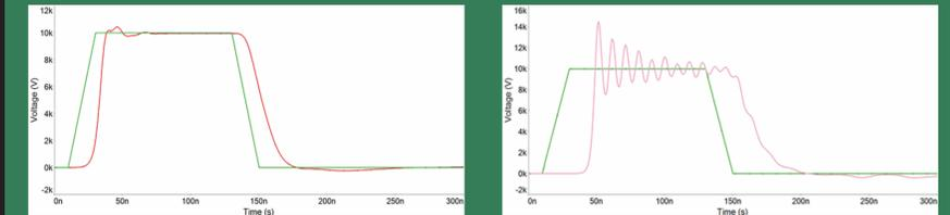
Spice model showing pulse sharpening from 16 ns to 8.4 ns (left). 100 MHz RF with lumped-element NLTL. Frequency can be changed by altering stray inductance.
