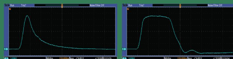
The next generation NLTL loads will be driven at higher voltage. EHT has demonstrated output pulses to 40 kV with 20 ns rise time and 40 - 130 ns pulse widths
