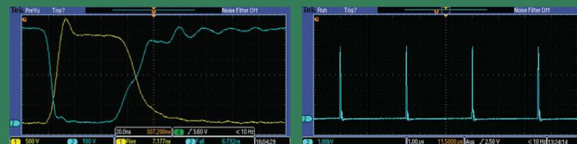
20 kV single pulse into 100  $\Omega$  load
