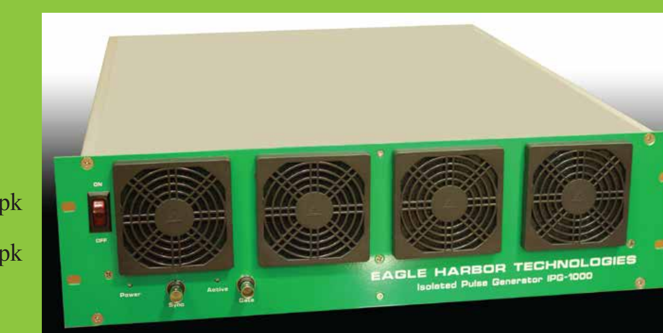
First generation EHT full-bridge pulser.
