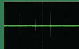
Left: NLTL RF output frequency as a function of magnetic bias field. Right: CVP output with 12.6 [kA/m] bias field. Burst of 4 pulses at 100 kHz. Horizontal scale 5  $\mu$ s/div, vertical scale 3333 V/div.
