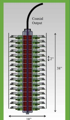
Design of 20 kV inductive adder that EHT is constructing.
