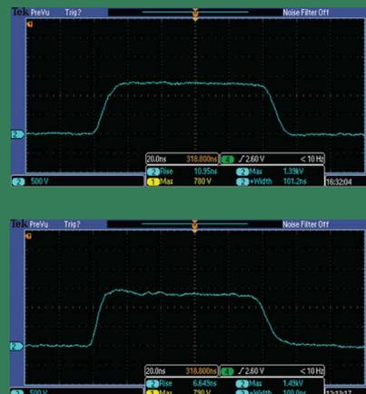
Left: 10 kV inductive adder. Top Right: 10 kV - 100 ns pulse into resistive 50  $\Omega$  load with 6.6 ns rise time. Bottom Right: 10 kV - 100 ns pulse into resistive 25  $\Omega$  load with 11 ns rise time.
