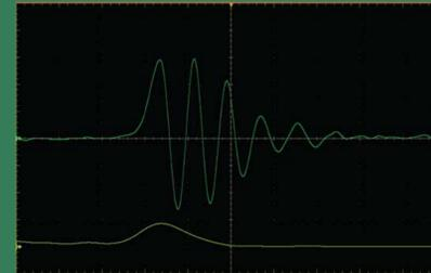
Left: Experimental setup showing the 50 Ohm pulse driver, the NLTL, and the CVP at the output of the NLTL. Right: CVP output (green) with 12.6 [kA/m] bias field. Horizontal scale 740 ps/div, vertical scale 3333 V/div. An FFT of the signal (yellow) has a peak at ~1.7 GHz. FFT scale is 25 mV/div vertical and 500 MHz/div horizontal.
