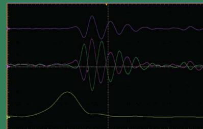
Left: Experimental setup with D-dot in far-field of monocone antenna. Right: From top to bottom signal names: Math 2, Ch3 (purple), Ch4 (green), Math4. Math2 = Ch3 - Ch4, Math4 = FFT(Math2). Vertical scale: Math2 = 2V/div, Math4 = 100mV/div, Ch3&Ch4 = 500 mV/div. Horizontal scale is 750 ps/div for signals and 500 MHz/div for FFT.
