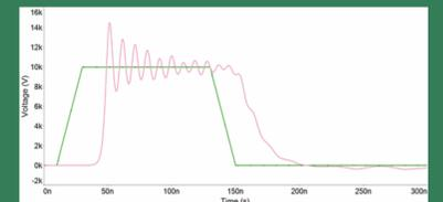
Left: SPICE model showing pulse sharpening from 16 ns to 8.4 ns. Right: 100 MHz RF with lumped-element NLTL.
