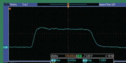
10 kV - 100 ns pulse into 25  $\Omega$  resistive load with 11 ns rise time.
