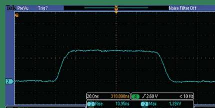
10 kV - 100 ns pulse into 50  $\Omega$  resistive load with 6.6 ns rise time.
