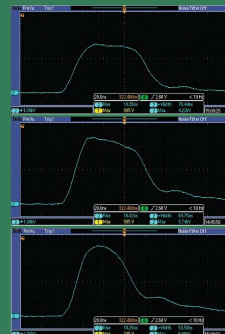
Output voltage pulses at 66 (top), 74 (middle), and 80 kV (bottom).
