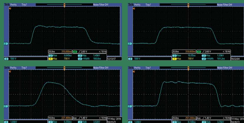
Top Left: 10 kV - 100 ns pulse into 50  $\Omega$  load with 6.6 ns rise time. Top Right: 10 kV - 100 ns pulse into 25  $\Omega$  load with 11 ns rise time. Bottom: 20 kV, 51 ns (left) and 110 ns pulse widths into 50  $\Omega$  load with 8.4 ns rise.
