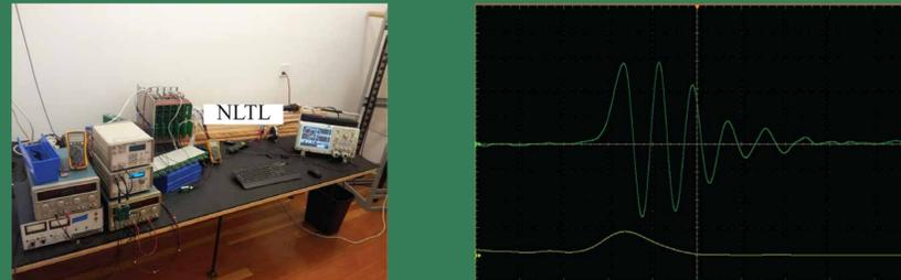
Left: Experimental setup showing the 50 Ohm pulse driver, the NLTL, and the CVP at the output of the NLTL. Right: CVP output (green) with 12.6 [kA/m] bias field. Horizontal scale 740 ps/div, vertical scale 3333 V/div. An FFT of the signal (yellow) has a peak at ~1.7 GHz. FFT scale is 25 mV/div vertical and 500 MHz/div horizontal.
