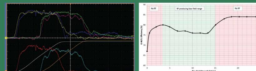
Left: Signals for G-NLTL single shot efficiency driving 52  $\Omega$  load at a bias field of ~17 kA/m. Input voltage (yellow), input current (blue), load voltage (purple), load current (green), instantaneous input power (red), instantaneous output power (cyan), total input energy (white), and total energy delivered to the load (orange). Efficiency is ~83%. Right: Coaxial NLTL broadband efficiency vs bias field strength.
