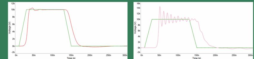
Spice model showing pulse sharpening from 16 ns to 8.4 ns (left). 100 MHz RF with lumped-element NLTL. Frequency can be changed by altering stray inductance.
