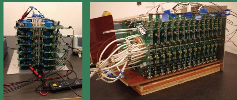
Left: 10 kV inductive adder. Right: 20 kV inductive adder.
