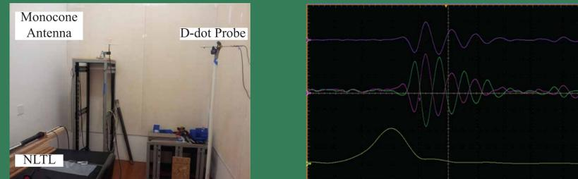
Left: Experimental setup with D-dot in far-field of monocone antenna. Right: From top to bottom: Math 2, Ch3 (purple), Ch4 (green), Math4. Math2 = Ch3 - Ch4, Math4 = FFT(Math2). Vertical scale: Math2 = 2V/div, Math4 = 100mV/div, Ch3&Ch4 = 500 mV/div. Horizontal scale is 750 ps/div for signals and 500 MHz/div for FFT.
