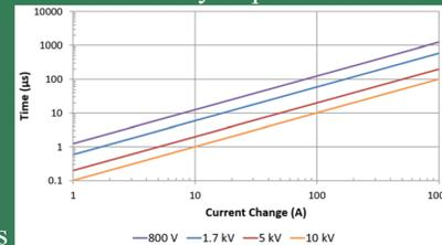
The time required to change the current in a coil with a 1 mH inductance.
