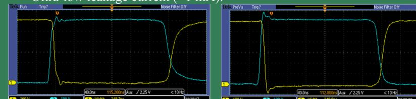
Oscilloscope traces showing rise and fall switching characteristics for both IGBTs (Left) and SiC MOSFETs (Right). Faster rise times are noted with the SiC MOSFETs.
