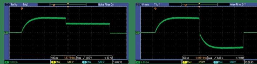
Left: Same as above right with a single negative going pulse at the transition for 7.8  $\mu$ s. Right: 2.15  $\mu$ s pulse width for 100 A for 1.5 ms followed by -100 A for 1.5 ms.
