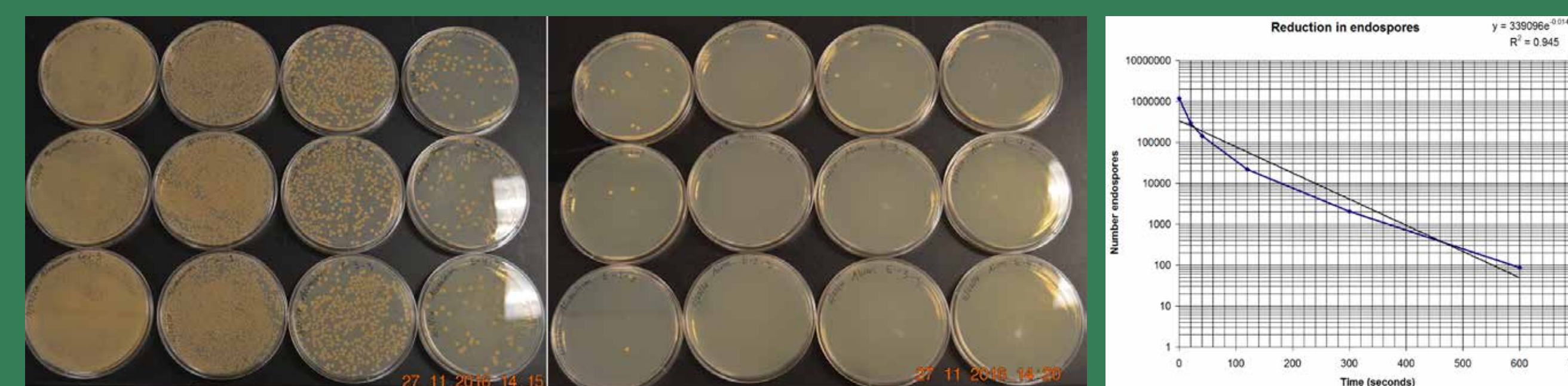
Left: Results of dilution series for control plates (left) and 10-min exposure (right). Columns represent 0.5 ml plated from dilutions of 1:10, 1:100, 1:1,000, and 1:10,000 (left to right). Rows represent triplicate plating of dilution series onto TSA. Plates were incubated for 24 hrs at 35 °C, with no more growth observed after 48-hour incubation.
