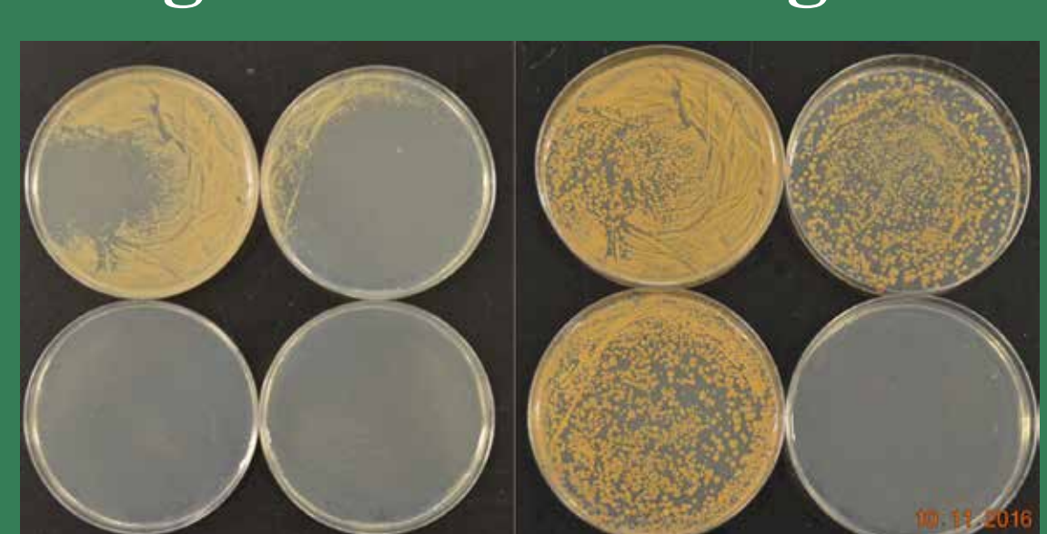
Jet passed over surface of Petri dishes containing 2.9 \times 10^7 endospores/ml for 1, 2, (top row), 5, and 10 min (bottom row). Results following 24-hr (left) and 48-hr (right) incubation at 35 °C. Only three colonies formed on the 10-min exposure, meaning jet achieved a 6 log reduction in endospores.
