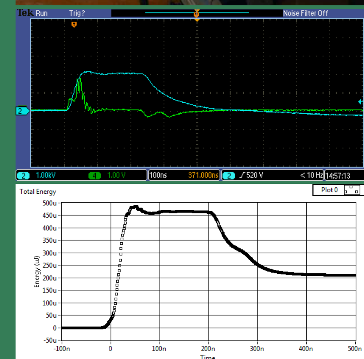
Top: Current (green) and voltage (blue) waveforms. Bottom: Energy per pulse.
