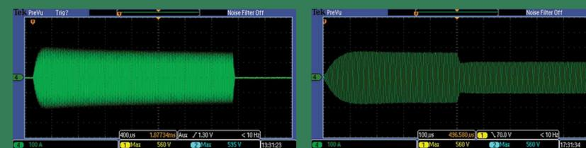
Resonant circuit: 85  $\mu$ H, 5 nF, and 1.25  $\Omega$  ( $f_{res} = 250$  kHz) Left: 200 A for 3 ms. Right: 500  $\mu$ s at 200 A and 500  $\mu$ s at 100 A. Both with 500 V drive.
