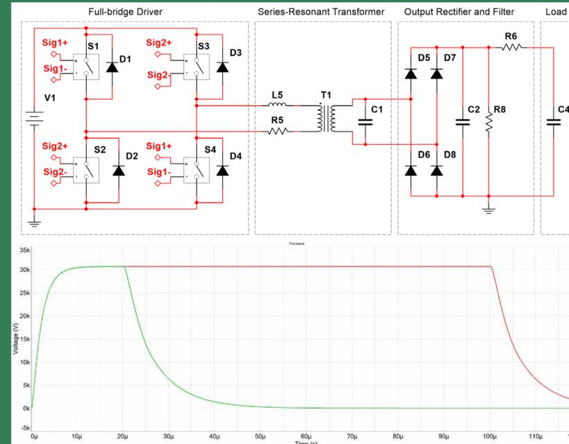
Top: Pulsar circuit diagram showing full-bridge, resonant circuit, rectifier and load. Bottom: Voltage across the load (C4) for 20 and 100  $\mu$ s pulses.
