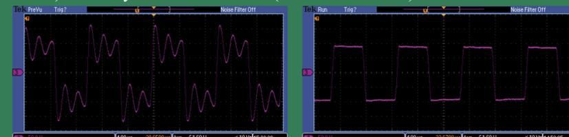
Waveforms showing Pre-Pulse off (left) and on (right). Circuit parameters: 50 W load, 10 mH of inductance, and 10 nF capacitance.
