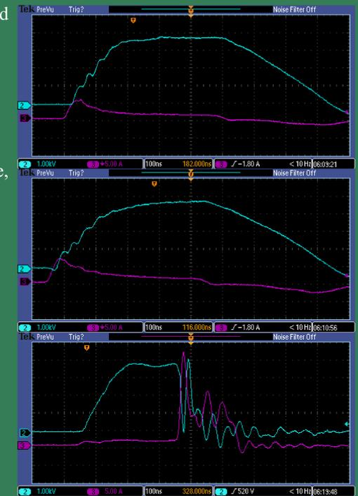
Output voltage (blue) and current (purple) waveforms for a 13 pF DBD (top), 35 pF DBD (middle), and arc (bottom).
