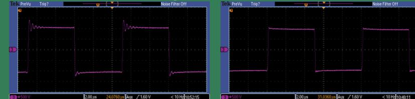
High voltage (10 kV) test showing Pre-Pulse off (left) and on (right).
