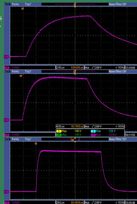
Single pulse waveforms: 30 kV with pulse widths of 10  $\mu$ s (top), 20  $\mu$ s (middle), 100  $\mu$ s (bottom).
