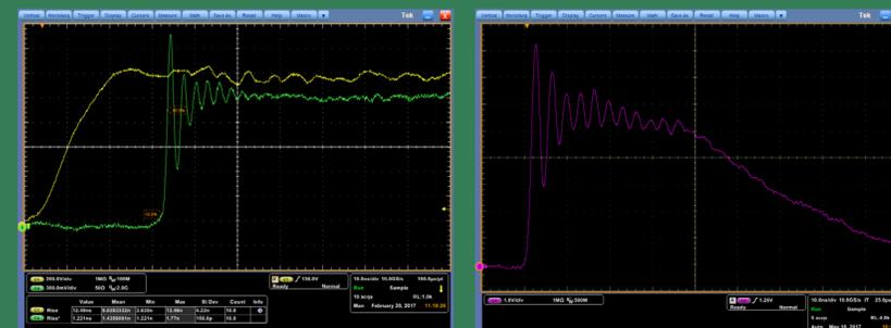
Left: Input pulse (yellow) and output pulse (green) from first generation RF NLTL. The frequency was 325 MHz, and about five oscillations were produced. Right: Output of second generation RF NLTL. The output frequency was 265 MHz and about double the number of oscillations.
