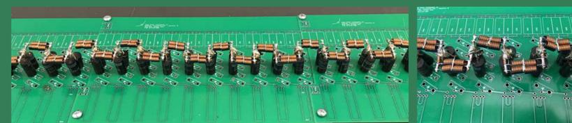
Left: Second-generation diode-based NLTL for RF production. Right: Close-up view of NLTL showing the new inductors.
