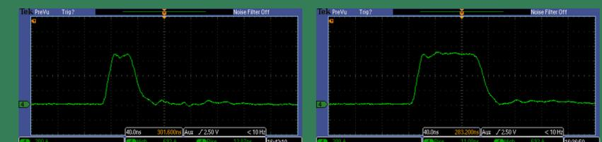
Inductive adder output measured by current monitor (Pearson 7713-03 with 1.5 ns usable rise time). Output was 35 kV into 50 Ω load. Pulse width was 40 ns (left) and 100 ns (right). Rise time 11-13 ns.
