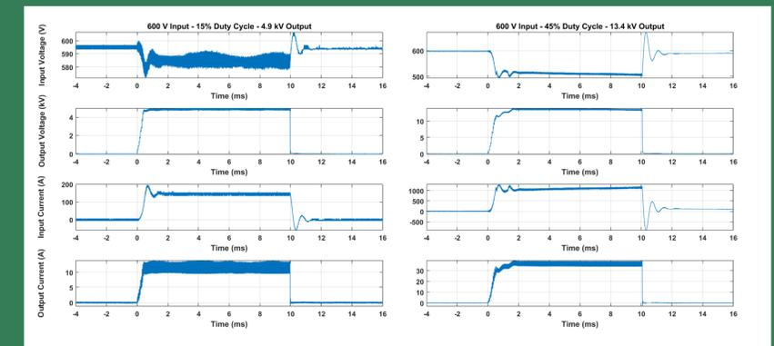
Plots of input and output voltage and input and output current with 600 V charge. Left: 15% duty cycle produced 4.9 kV into 357  $\Omega$  load. Right: 45% duty cycle produced 13.4 kV into 375  $\Omega$  load.
