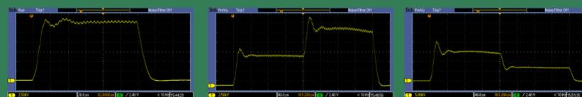
Left: 15 kV output for 120  $\mu$ s into 375  $\Omega$  load. Middle: Increasing the voltage from 7.5 kV to 15 kV by increasing the duty cycle. Right: Decreasing the voltage from 15 kV to 7.5 kV by decreasing the duty cycle.
