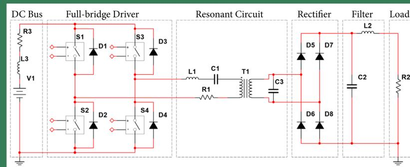
Simplified Multisim circuit model. Actual circuit model included stray components.
