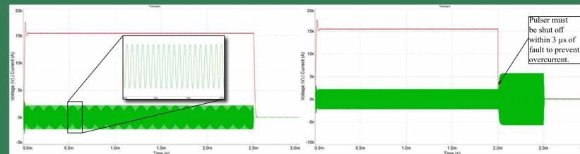
Left: Load voltage (red) and oscillating current (green) during normal operation. Initial voltage spike can be eliminated by lowering the switching duty cycle during startup. Right: Simulation of load fault at 2 ms. System must be shut down with 3 ms of fault to prevent overcurrent of solid-state switches in the full-bridge driver.
