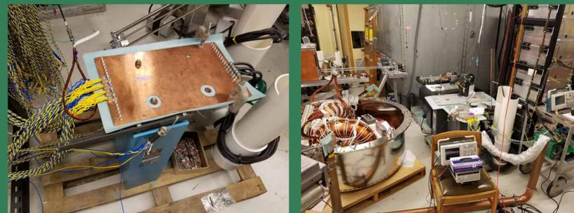
Left: Resonant capacitors, tuning inductors, and Rogowski coil. Right: Single EHT SPA board connected to resonant load with helicity injectors shown.
