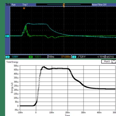
Top: Current (green) and voltage (blue) waveforms. Bottom: Energy per pulse. L: 2.5 cm, 12 kV, 20 ns, 6 kHz, 16 LPM R: 6.2 cm, 12 kV, 220 ns, 4 kHz, and 4 LPM
