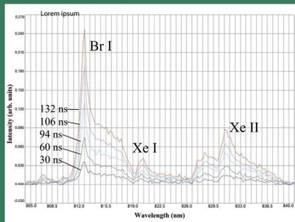
Left: 106 ns (top) and 132 ns (bottom) pulses deposited 1.2 mJ and 1.4 mJ into the plasma, respectively. Right: While increases in the blackbody radiation were modest, Br I, Xe I, and Xe II spectral lines increased dramatically with pulse width. This indicates potential utility of nanosecond pulsers in excimer production
