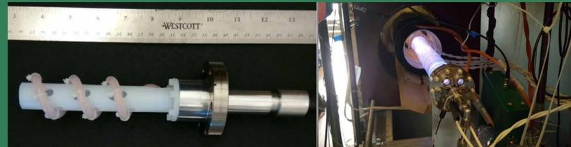
Left: HPRF antenna side view. Right: Electrodeless plasma source during operation.
