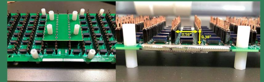
Diode-based NLTL was constructed with 30 kV unencapsulated diodes to act as the nonlinear capacitors. Off-the-shelf inductors were used to simplify construction.
