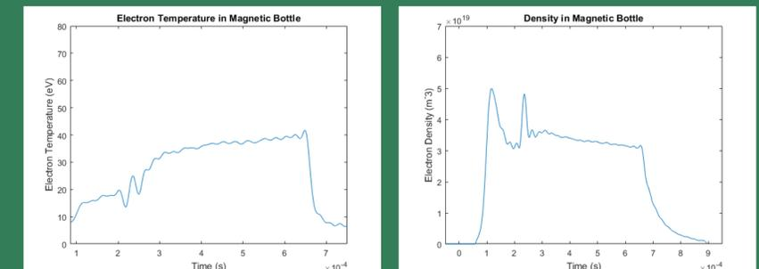
Left: Electron temperature as a function of time as measured near the low point in the magnetic bottle. Right: Plasma density as a function of time at the same location.
