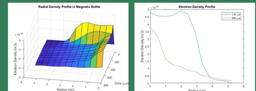
Left: Radial profile of electron density as a function of time. Right: Radial electron density profile at two time slices. Plots show initial ionization followed by a compression of the plasma profile into a narrow beam.
