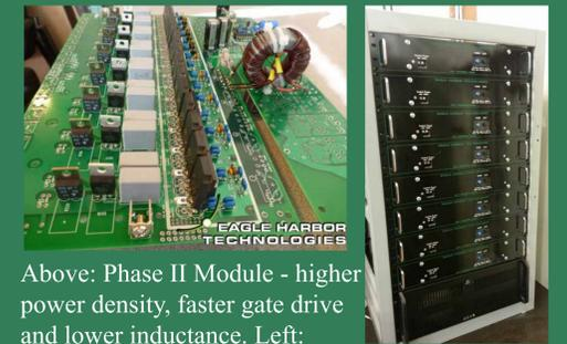
Above: Phase II Module - higher power density, faster gate drive and lower inductance. Left: IPMs operated in parallel to switch 40 kA.
