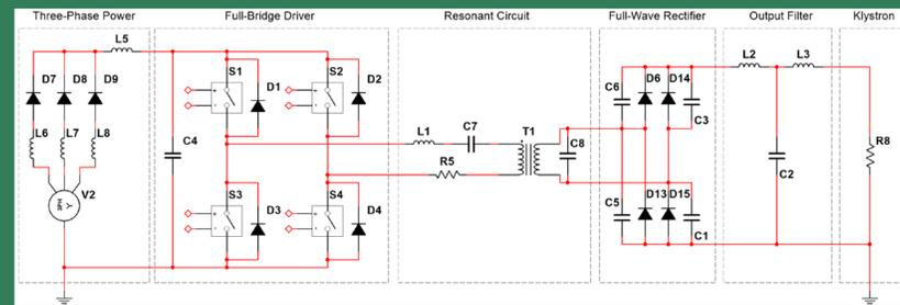
Simplified Multisim circuit model. Actual circuit model included stray components.
