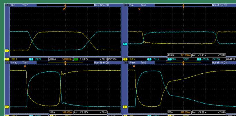
Switching waveforms at 600 V and 20 A with 10 Ω gate resistor. Top left: Standard. Top Right: APT25GR120BD15. Bottom Left: FGH12040WD-F155. Bottom Right: STGWA40N120KD.
