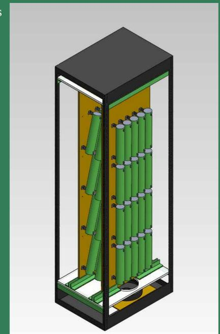
30 kW load resistor CAD model.
