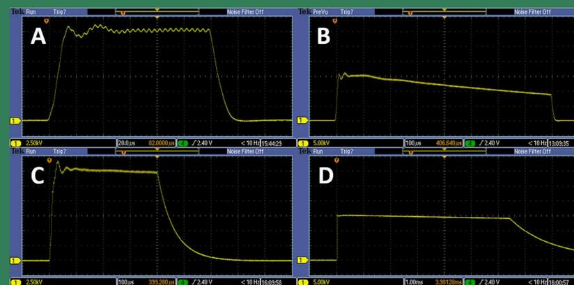
15 kV pulses with varying shot lengths and loads. A: 375  $\Omega$  and 120  $\mu$ s, B: 375  $\Omega$  and 800  $\mu$ s, C: 4.4 k $\Omega$  and 400  $\mu$ s, D: 100 k $\Omega$  and 7.5 ms.
