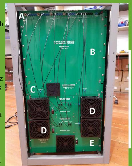
HV power system of the NBI. The front panels of A: FT4x4, B: step-up output module, C: HVIM fault monitor, D: two SPAs running in parallel, and E: the ACIM.
