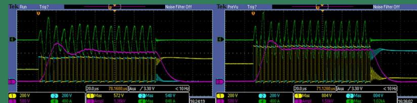
Characteristic waveforms showing 10 kV output into 375  $\Omega$ . Left is a shot with a charge voltage of 450 V and a duty cycle of 75% and right has an increased charge voltage of 650 V and a lowered duty cycle of 60%. Ch1 and 2 (yellow and blue) are the voltages across the switch. Ch 3 (magenta) is the output voltage measured by a 1:7 voltage divider. Ch 4 (green) is the circulating current out of the SPAs.
