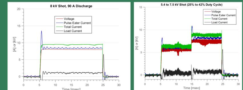
Operation with neutral beam grids Left: 8 kV shot showing ~1 A of beam current through the acceleration grid. Right: Dynamic control of voltage output of the NBI system at the user's facility during plasma shots (right).
