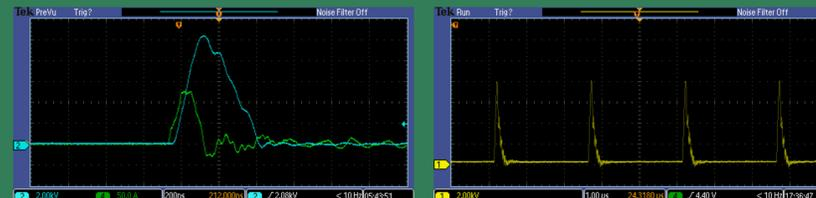
Left: The voltage (green) and current (blue) waveforms into 1 nF load from a 10 kV pulse with 100 ns rise time. Right: The waveform shows 9 kV pulses with 40 ns rise time repeating at 400 kHz into a 600 pF load.
