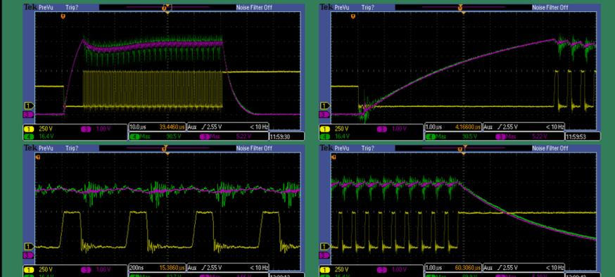
IPMs operated at 600 V, 350 ns pulse width, for 120 pulses at 2 MHz. Flattop current is 2.0 kA. Traces shown are  $V_{cc}$  (yellow), current probe (pink), and shunt resistor (green).
