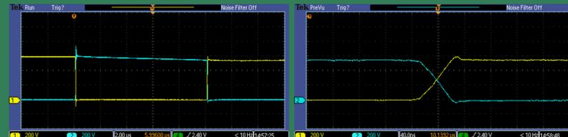
Left: Clean switching waveform into 1  $\Omega$  load. Right: Same waveform showing fast voltage and current rise time (< 40 ns).
