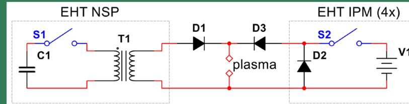
Circuit diagram showing the EHT NSP and four EHT IPMs connected to an arc system. D1 and D3 are isolation diodes that prevent high current from flowing into the NSP and high voltage from being generated on the IPMs.
