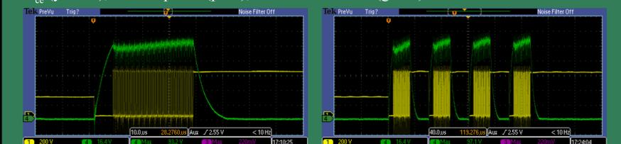
IPMs operated at 600 V with a pulse width of 375 ns for 240 pulses which produced flat top currents of 2.0 kA. Single burst (left) and four bursts at 17 kHz (right). Traces shown are  $V_{cc}$  (yellow) and shunt resistor (green).
