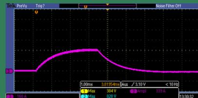
Left: EHT IPM Right: Current waveform. IPM driving a 85  $\mu$ H inductor at 350 V and 340 A with a PWM drive frequency of 30 kHz.
