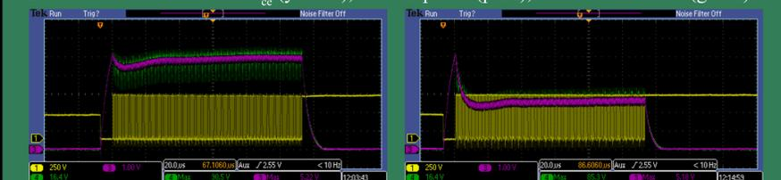
IPMs operated at 600 V for 240 pulses with a pulse width of 350 ns (left) and 200 ns (right), which produced flat top currents of 2.0 kA (left) and 1.1 kA (right). Traces shown are  $V_{cc}$  (yellow), current probe (pink), and shunt resistor (green).
