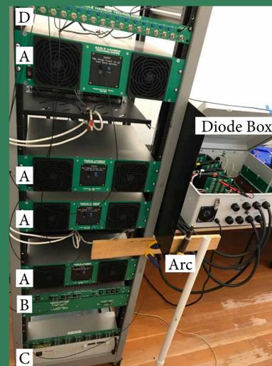
Left: Rack containing four EHT IPMs (A), charge dump system (B), DC charging supply (C), and fiber optic trigger system (D). Right: Plasma arc.
