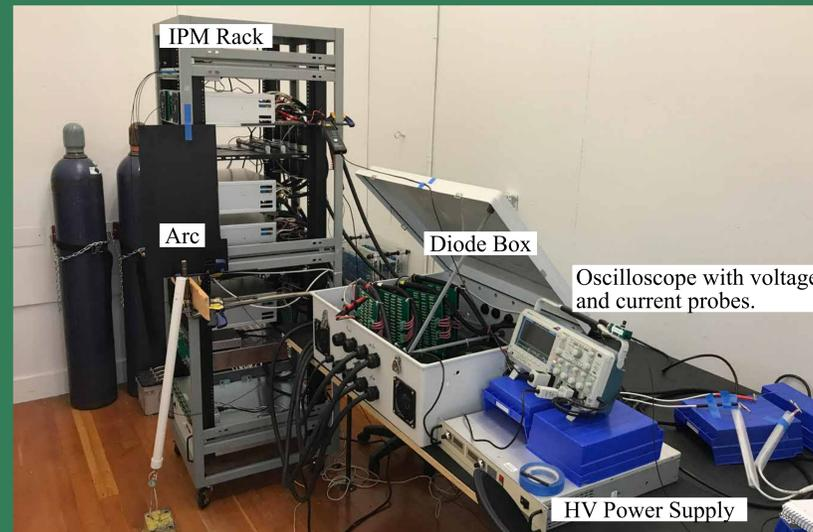
Experimental setup showing IPM rack, arc, diode box, high voltage power supply, and oscilloscope.
