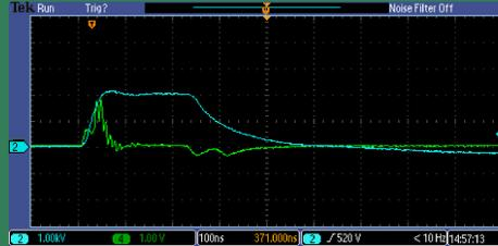
Left: EHT NSP-120-20-P-500. Right: Voltage (blue) and current (green) measurements of a dielectric barrier discharge driven by the NSP.
