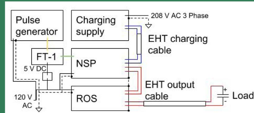
Block diagram of the NSP-RCC integrated into larger system.
