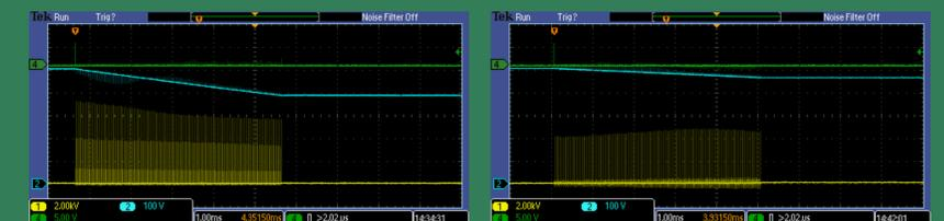
Energy recovery testing. Voltage droop on energy storage capacitors (blue trace), output voltage (yellow), and trigger (green) without (left) and with (right) energy recovery implemented.
