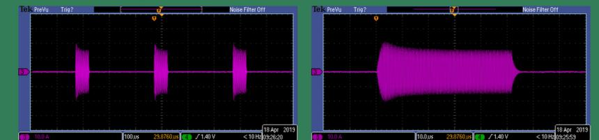
Antenna current with plasma production at 13.56 MHz. Left: 50  $\mu$ s burst with 300  $\mu$ s burst repetition frequency. Right: Expanded timescale of a single RF burst.
