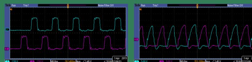
Left: Input signal from BNC inputs for the two channels. Right: Gate signal at input to the GaN HEMTs.
