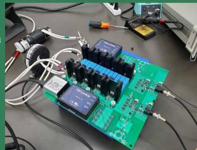
EHT half-bridge with GaN HEMTs driving a series resonant circuit.
