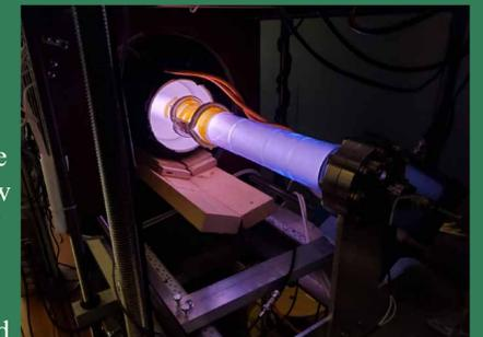
Hydrogen plasma produced with matchless RF generator driving an inductive antenna.
