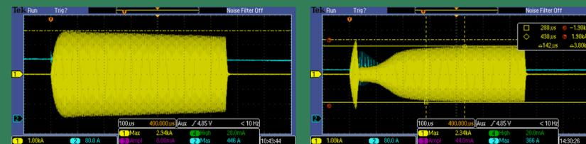
Antenna current for a vacuum shot (left) and plasma shot (right). The flat top current is 2.94 kA and 1.9 kA for the vacuum and plasma shots, respectively.
