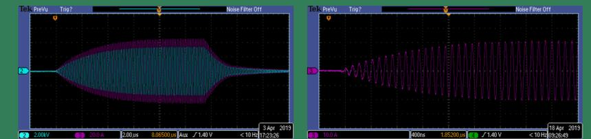
Antenna current without plasma at 13.56 MHz. Left: 12  $\mu$ s burst 45 A of current in the antenna. Right: Expanded timescale showing the rise of the RF burst.
