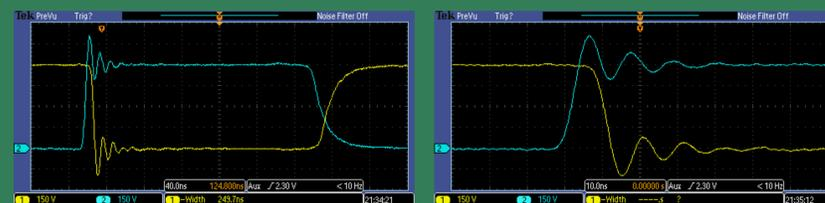
Measurement of switch voltage (yellow) and current (blue) of an IGBT at EHT at two different timescales. The IGBT was operated at 600 V and 12 A. The rise time was 4 ns.
