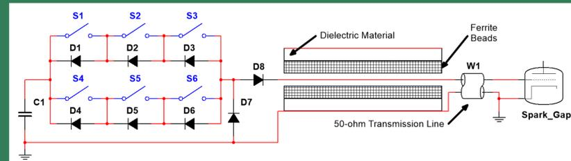
Circuit diagram of proposed series/parallel arrangement of switches with NLTL
