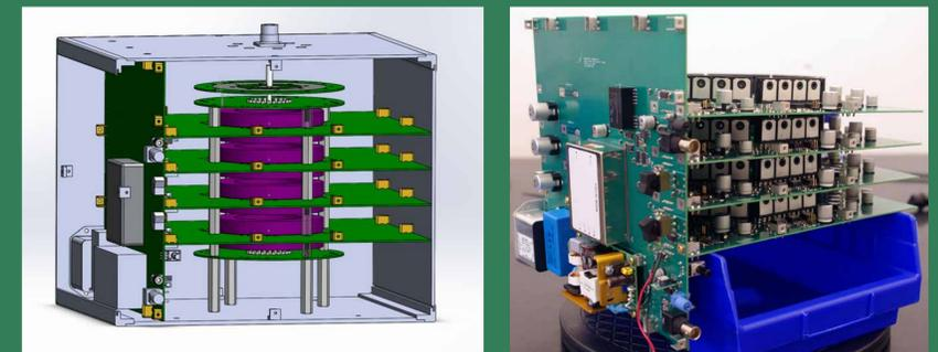
Left: CAD model of inductive adder in enclosure. Right: Four-board inductive adder stack with control board mounted on left side.
