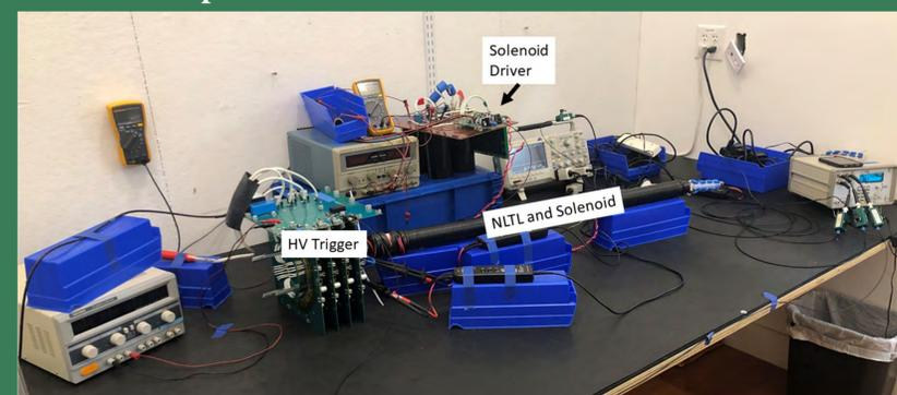
High voltage test setup for the HV Trigger based on the inductive adder and NLTL.
