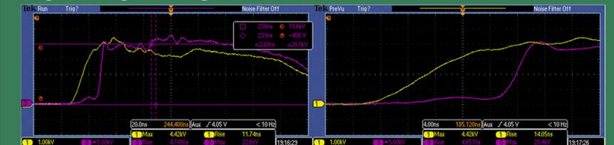
The transformer output (yellow) and NLTL output across the 50  $\Omega$  load (magenta) with 20 ns/div (left) and 4 ns/div (right). The cursors in the left image indicate 20 kV. NLTL solenoid bias magnetic field was 29 kA/m, DC charge voltage of 950 V.
