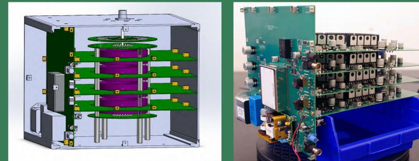
Left: CAD model of inductive adder in enclosure. Right: Four-board inductive adder stack with control board mounted on left side.
