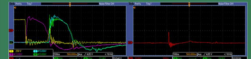
HV Trigger driving a 0.15" spark gap at the end of the delay line (left) and spark gap voltage (right).  $V_{CE}$  (yellow), voltage across 50  $\Omega$  resistor in series with the spark gap (blue), output voltage of the transformer (magenta), the voltage across the spark gap and 50  $\Omega$  series resistor (green), and spark gap voltage.
