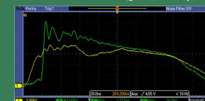
HV Trigger with second NLTL design driving 50  $\Omega$  resistor. This NLTL did not require an external magnetic field, but produced 30 kV with a sub-3 ns rise time. Inductive adder output (yellow) and NLTL output (green).
