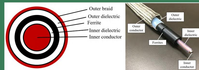
Ferrite-based NLTL design cross-sectional (left) and constructed NLTL (right).
