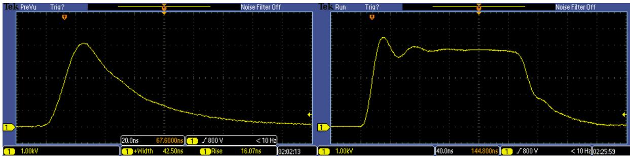
**Figure 13.** Minimum (left) and maximum pulse widths at 20 kV.
