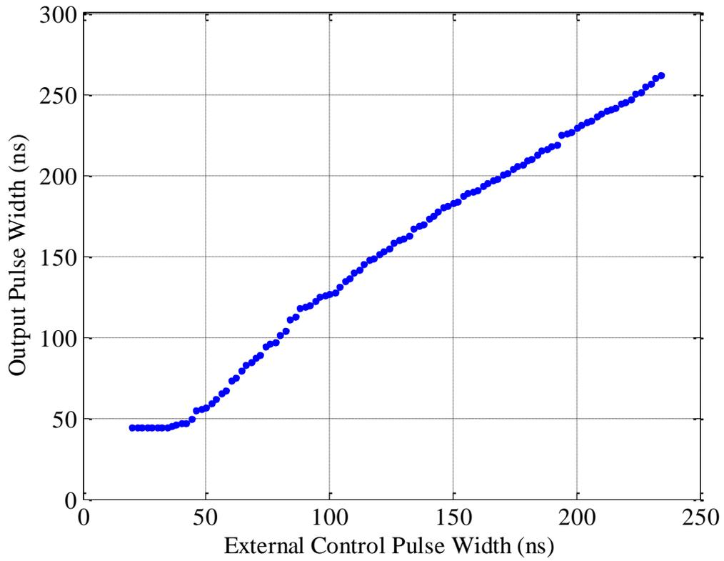
**Figure 9.** Input pulse width vs output pulse width for NSP-120-20-F
