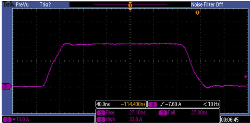
**Figure 25.** Maximum pulse width on a shorted output, demonstrating the maximum  $dI/dt$  and current for the unit (1.2 A/ns up to a flat-top of approximately 33 A).
