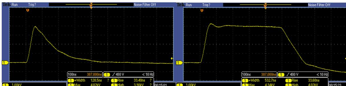
**Figure 23.** Minimum (left) and maximum pulse width voltage across a 10 kΩ 1:5 resistive voltage divider.
