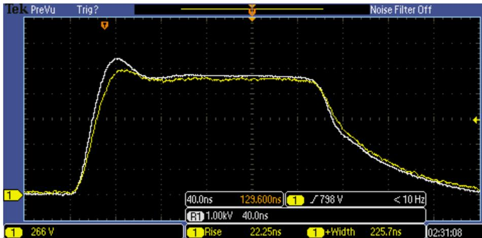
**Figure 14.** Comparison of internal voltage divider (white) with 1 pF capacitive voltage divider (yellow).
