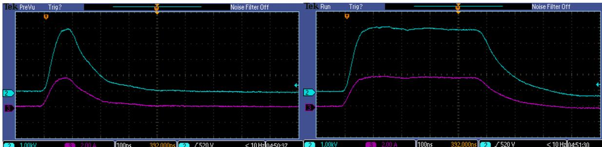
**Figure 18.** Voltage (blue) and current (purple) for minimum (left) and maximum pulse widths across a 2.5 kΩ 1:9 resistive voltage divider.
