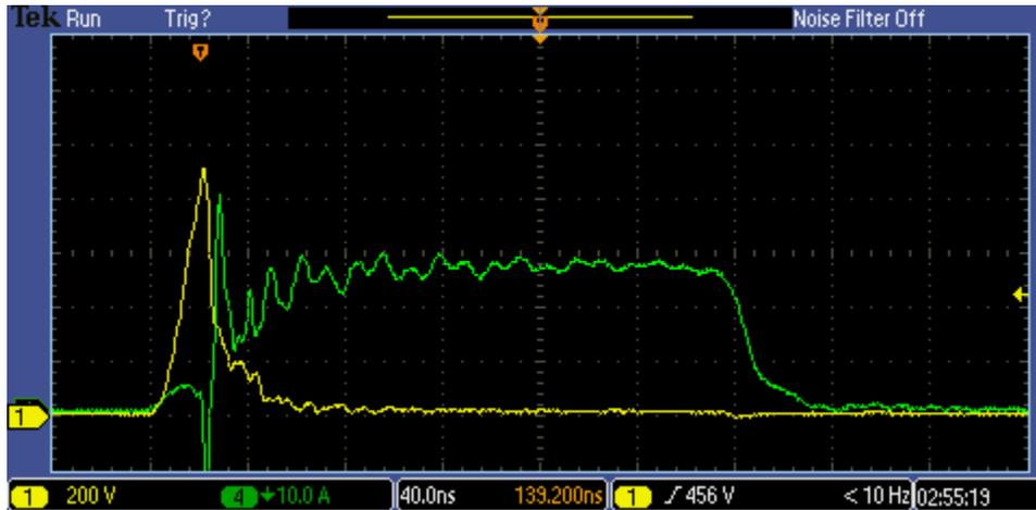
**Figure 17.** Load voltage (yellow) and current (green) for an arc and a 1 pF voltage divider.
