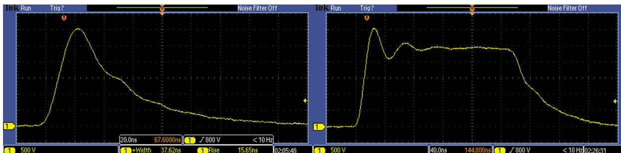
**Figure 12.** Minimum (left) and maximum pulse widths at 10 kV.
