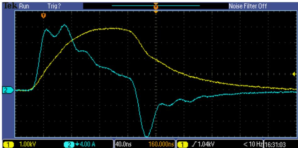
**Figure 16.** Load voltage (yellow) and current (blue) for a 35 pF DBD with a 5 kΩ voltage divider.
