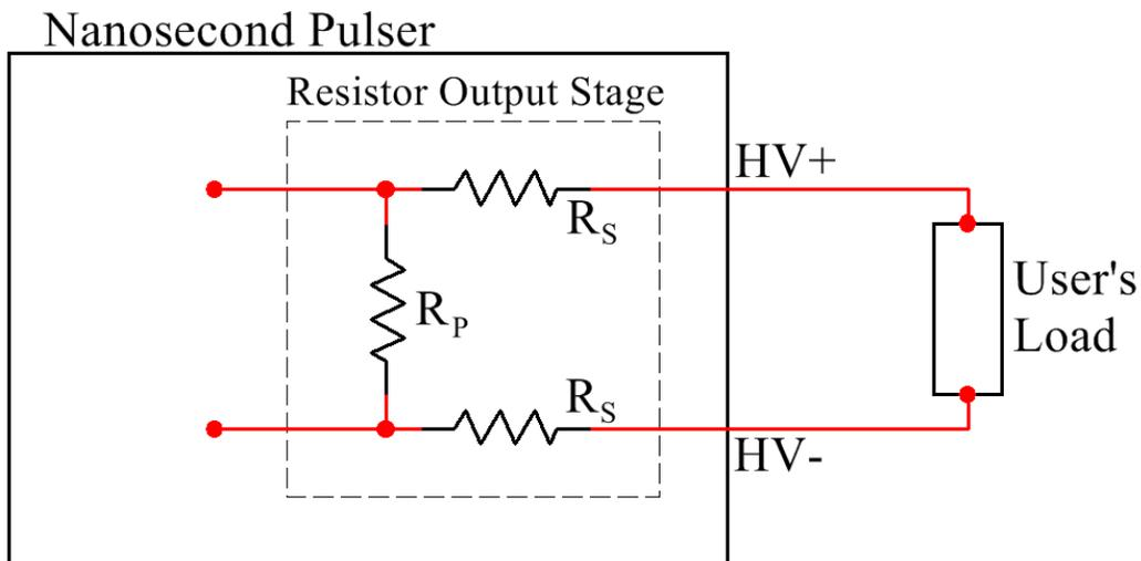
**Figure 5.** Resistive Output Stage for Floating Units
