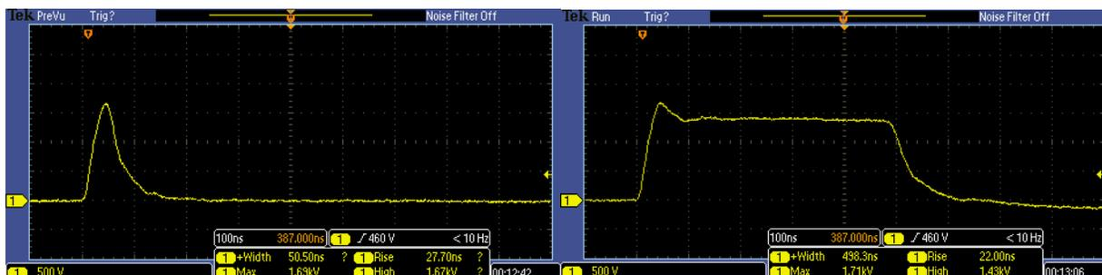
**Figure 22.** Minimum (left) and maximum pulse width voltage across a 1 kΩ 1:9 resistive voltage divider.
