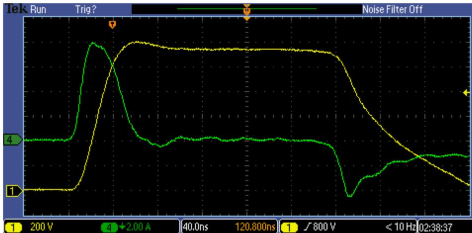
**Figure 15.** Load voltage (yellow) and current (green) for an 8 pF DBD and a 1 pF voltage divider.
