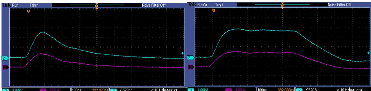
**Figure 19.** Voltage (blue) and current (purple) for minimum (left) and maximum pulse widths across a 10 kΩ 1:9 resistive voltage divider.
