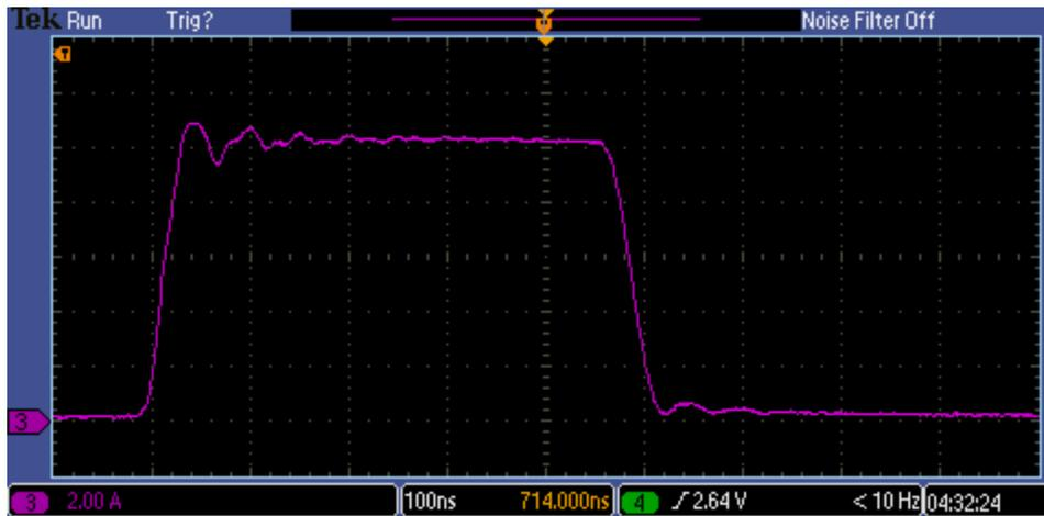
**Figure 21.** Maximum pulse width on a shorted output, demonstrating the maximum  $dI/dt$  and current for the unit (1.1 A/ns up to a 34 A peak with a flat-top of approximately 30 A). Please note that the vertical scale reported by the oscilloscope is incorrect.
