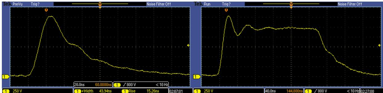
**Figure 11.** Minimum (left) and maximum pulse widths at 5 kV.
