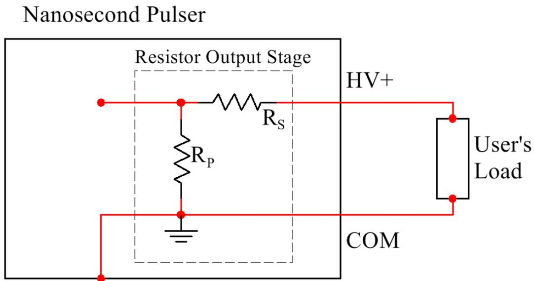
**Figure 6.** Resistive Output Stage for Grounded Units
