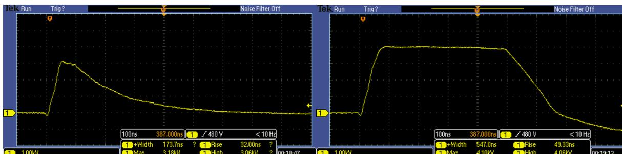
**Figure 24.** Minimum (left) and maximum pulse width voltage across a 10 pF 1:5 capacitive voltage divider.
