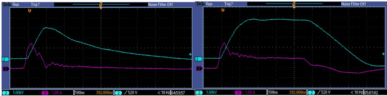
**Figure 20.** Voltage (blue) and current (purple) for minimum (left) and maximum pulse widths across a 10 pF 1:9 capacitive voltage divider.
