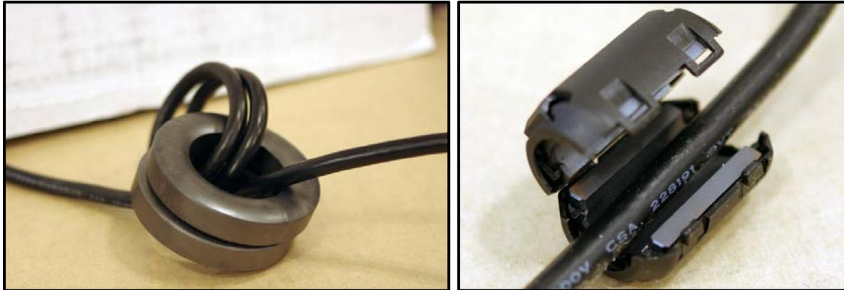
(Left) Cable wrapped loosely around two ferrites. (Right) Cable passed through a ferrite clamp.
