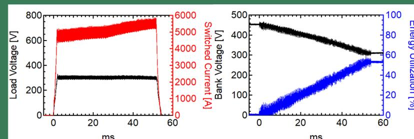
Ćuk module operating at the design specification. Left: output voltage (black) and total switch current (red). Right: Capacitor bank voltage (black) and percent of energy utilized from the capacitor bank (blue).
