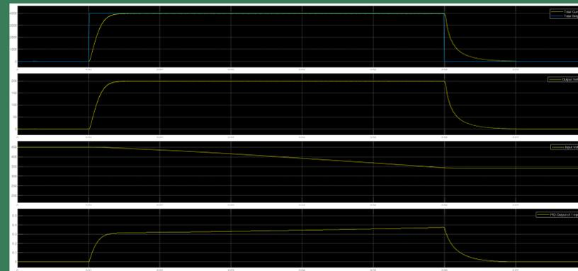
MATLAB/SIMULINK results two Ćuk modules operating in parallel for the arc circuit (from top to bottom): output current, output voltage, input voltage, and PI output.
