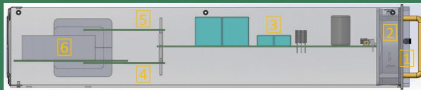
Side view of the second generation Ćuk converter full module showing the input fiber (1), cooling fans (2), Ćuk switching components (3), input current limiter board (4), output current limiter board (5), and AC isolation transformer (6).
