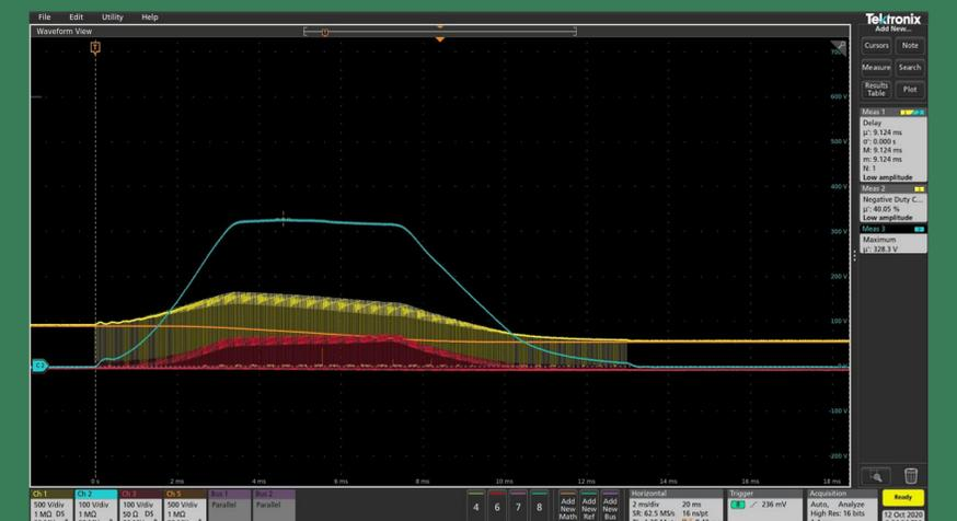
Small-scale Ćuk module operating with real-time PI controller: output voltage (blue), Vcc (yellow), capacitor bank voltage (orange), switch current (red).
