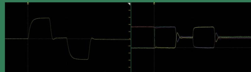
Output voltage measured across a 70  $\Omega$  load (left) and  $V_{ce}$  measurements of all four switching positions (right - yellow is position 1, blue is position 2, red is position 3, green is position 4). 3 kV charge, 1  $\mu$ s pulse width for both the positive and negative pulse, 1  $\mu$ s dwell time between pulses.
