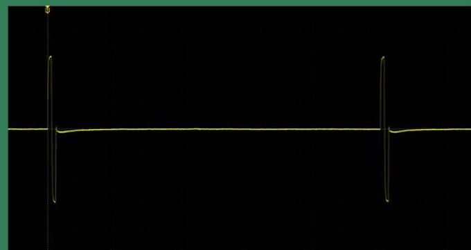
Output voltage measured across a 70  $\Omega$  load, 3 kV charge, 1  $\mu$ s pulse width for both the positive and negative pulse, 100 ns dwell between pulses, two pulses at 10 kHz PRF.
