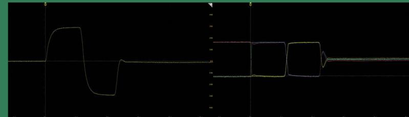
Output voltage measured across a 70  $\Omega$  load (left) and  $V_{ce}$  measurements of all four switching positions (right - yellow is position 1, blue is position 2, red is position 3, green is position 4). 3 kV charge, 1  $\mu$ s pulse width for both the positive and negative pulse, 100 ns dwell time between pulses.
