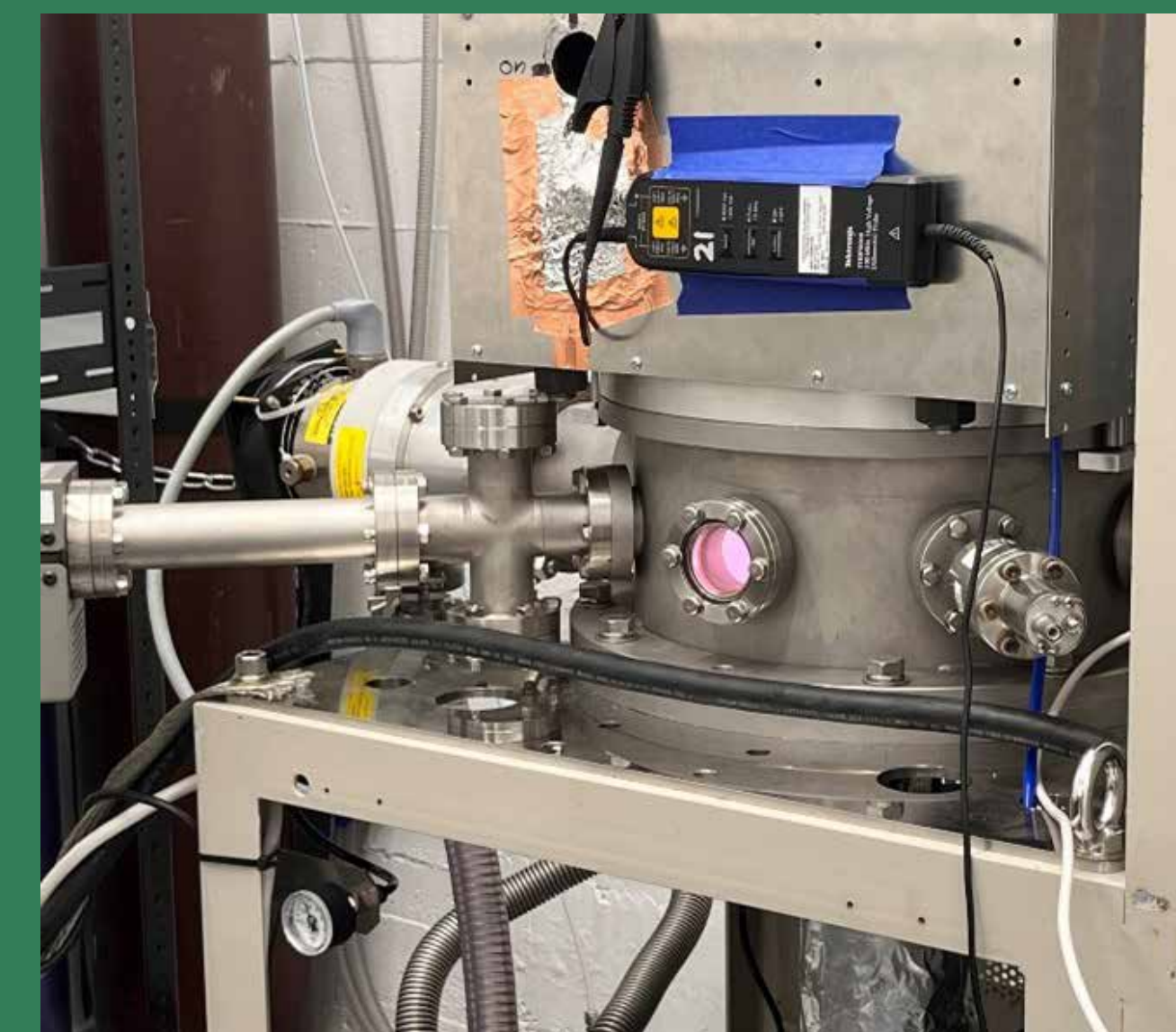
Argon plasma produced by a 60 MHz CCP with high voltage probe measuring the RF.
