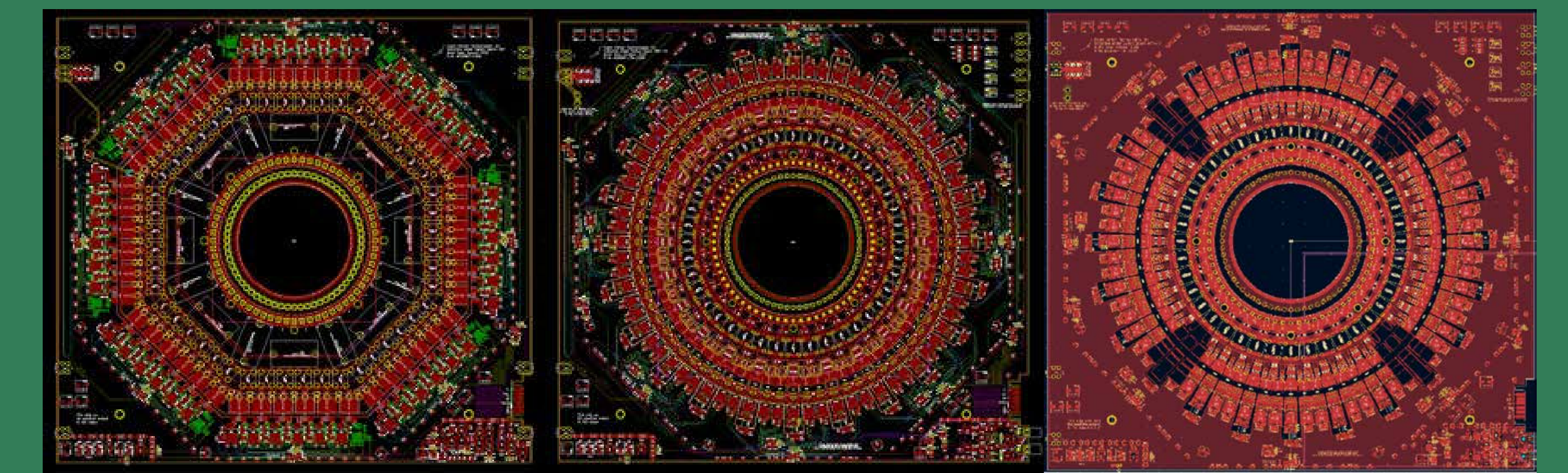
Comparison of EHT inductive adder PCBs: original design (left), Phase I design (middle), Phase II design with new SiC MOSFETs.
